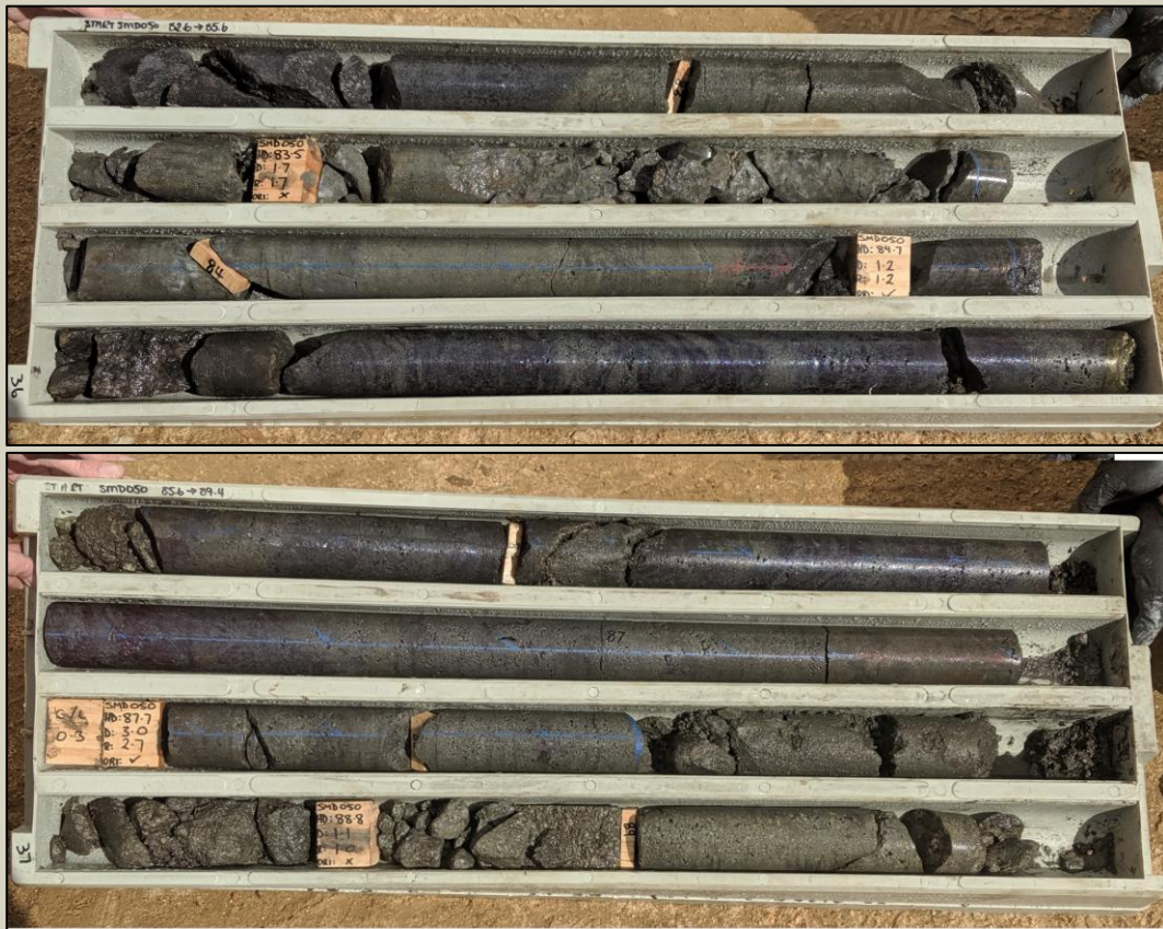
Photos 1 & 2. Massive sulphide interval from 82.6m to 89.4m drill depth in SMD050. Note the purple mineral is bornite.
