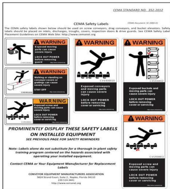
FIG: Shows various warning label as CEMA 352-2012
