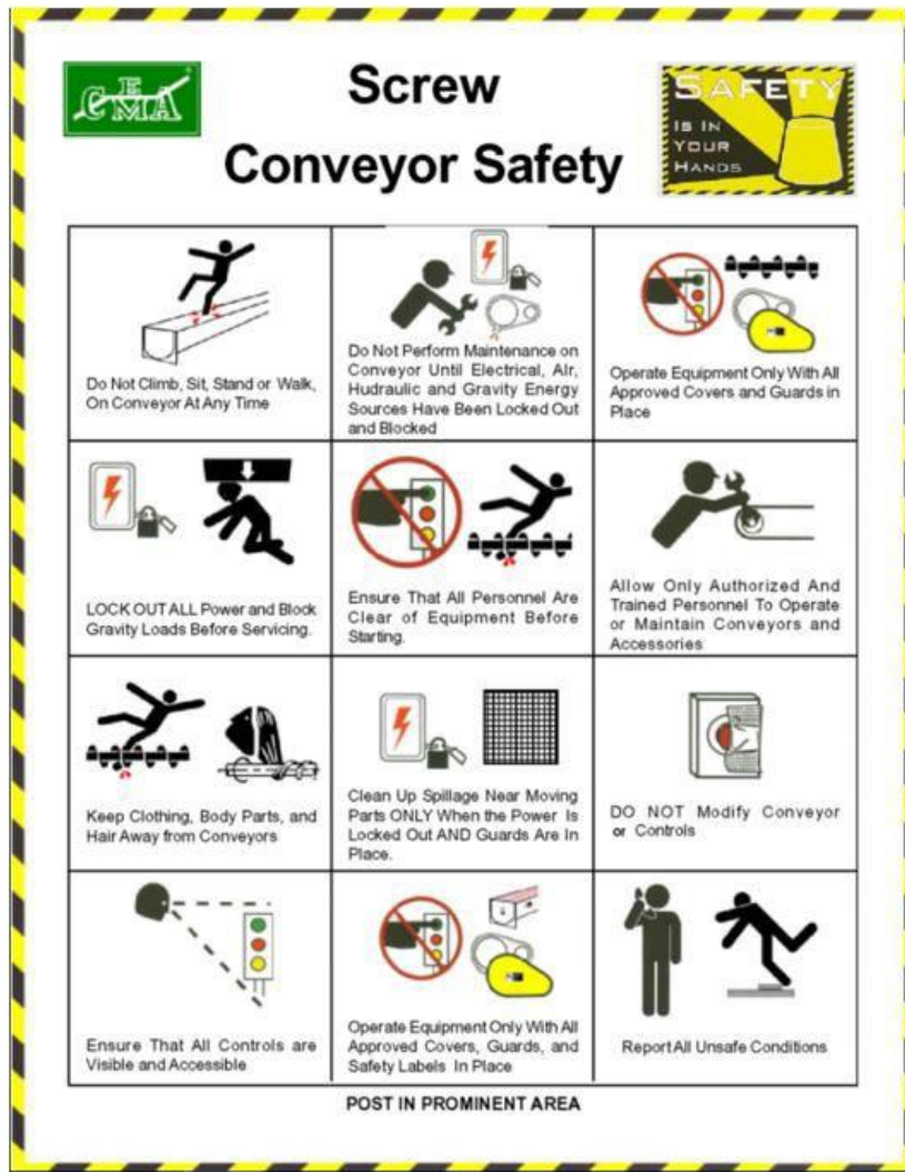
FIG: Shows some general Screw Conveyor Safety Labels as CEMA
