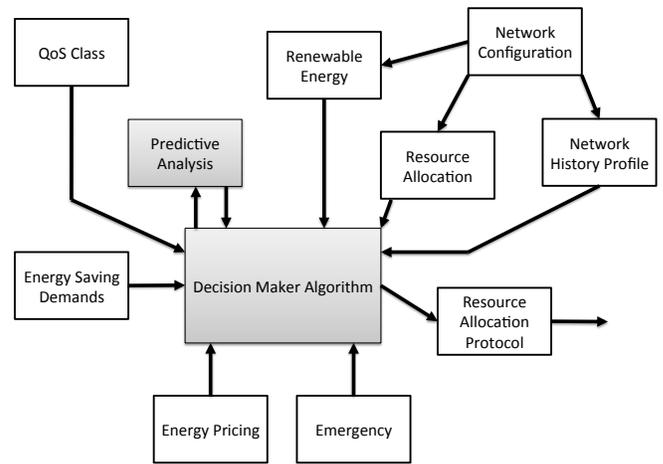
Fig. 3: Closer look at the EE protocol. Nine elements give relevant input information for a decision maker algorithm set up a desire resource allocation configuration. Machine learning components are in grey.
