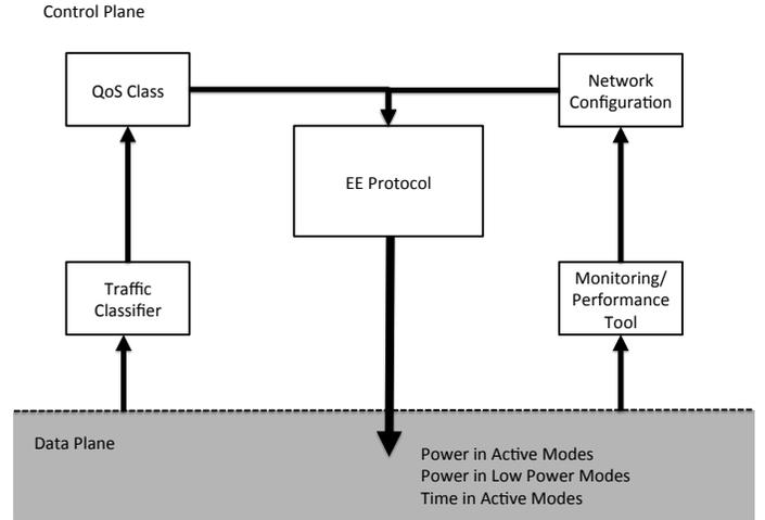
Fig. 2: Control plane accommodates the energy efficiency architecture (EEA) in a 5G platform. The EEA have inputs from the control plane that process data acquired from the data plane
