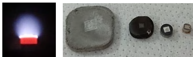
Fig. 1 (left) 3x3 mm <100> diamond substrate at the centre of the susceptor surrounded by the CVD plasma during growth. (right) Different sizes of pedestals that were used during the growths. Sizes ranges from ~24mm to 4.30mm.
