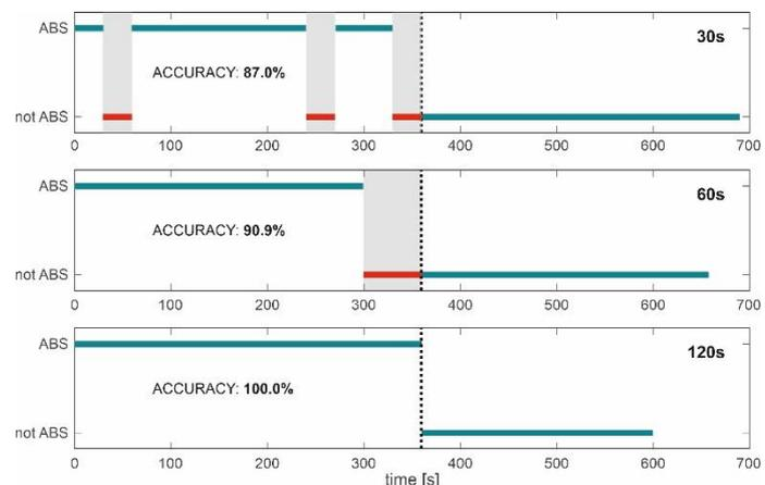
**Figure 6.** Automatic detection for two faulty samples: filament absent 6 minutes after the start (top row), ABS filament misplaced with PLA 6 minutes after the start (bottom row). Incorrectly detected segments are marked as shaded regions.
