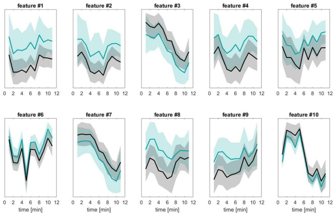
**Figure 4.** Separation between the best ranked features extracted for ABS and two other cases (PLA+NF) across the time. The mean±std are marked with green (ABS) and black (PLA+NF) solid line and shaded areas respectively.
