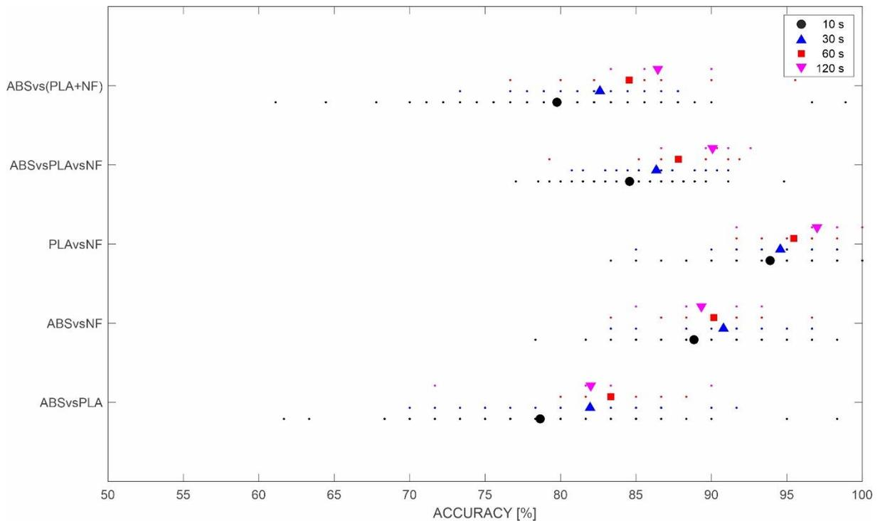
**Figure 5.** Accuracy of the ML system for different lengths of data segments and datasets (average values across all segments are presented with markers in different colours)
