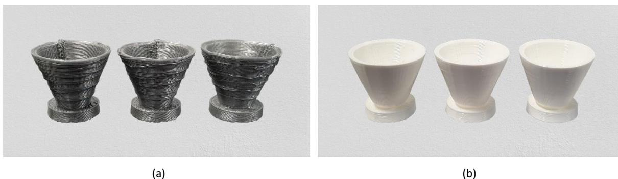
**Figure 2.** Samples printed using two different filament types: (a) ABS and (b) PLA
