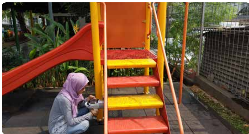
Figure 7. Staff of Nexus3 Foundation measuring lead content in playground facilities using portable XRF analyser. Photo: Nexus3 Foundation
