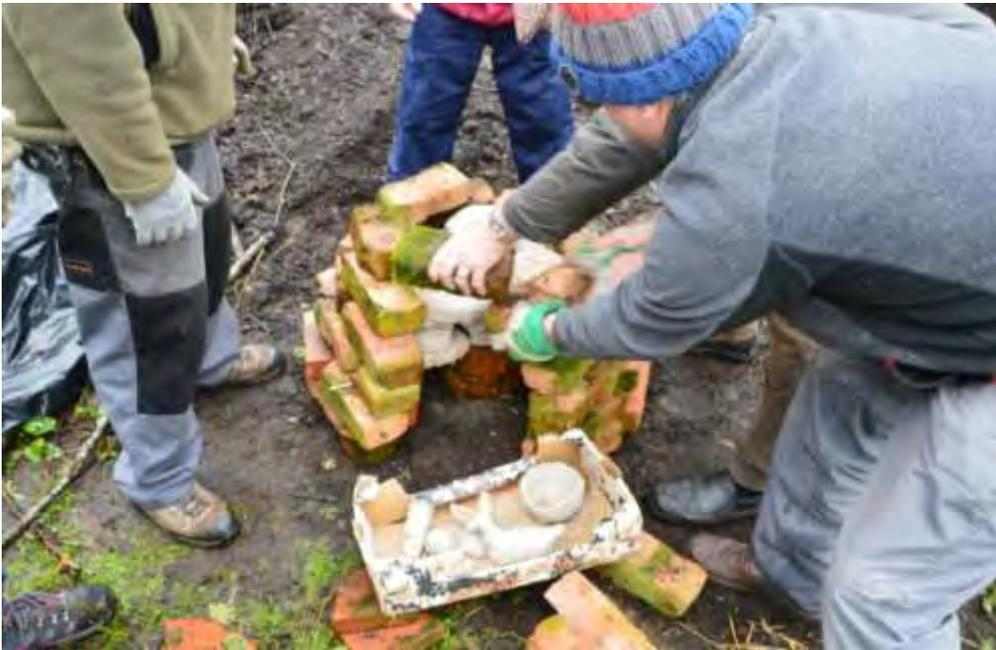
Using old household bricks and quarry tiles we built a round construction with a opening at the front. As it was built we loaded it with the pots and objets d'art. There was a column in the centre to try to raise the pots etc of the ground and allow the hot air to flow around and through the kiln.
