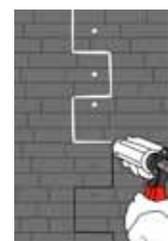
Once the surface is all covered with panels fill in assembly joints and drilled holes with the putty.
