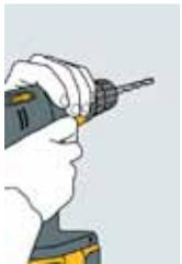
Remove the panel and drill with the 8mm bit where the wall has been previously marked with the 3mm bits
