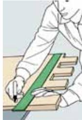
Use a ruler and a marker and draw a line along the surface to be cut.
