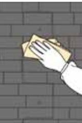
Right after when the paint is still wet rub a wet cloth over the joints to cover the pores. Do it as many times as needed.
