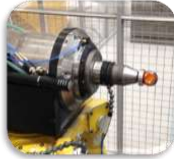
(b) Robot with SMR attached
