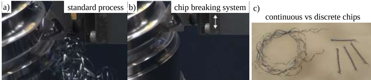
Figure 6: Chip formation for standard and chip breaking processes.
