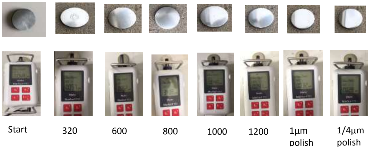
Figure 10: Stages in Grinding and Polishing
