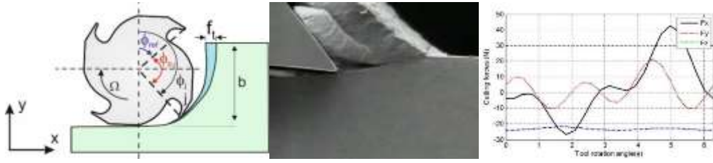
Figure 11: Effect of feed rate fluctuations on chip formation and cutting forces.
