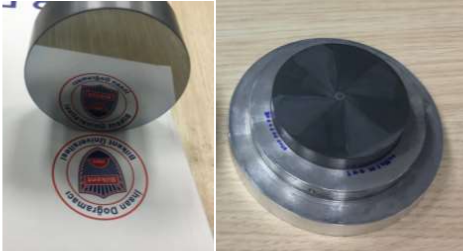
Figure 14: a) Finished silicon surface, b) machined with worn diamond tool.
