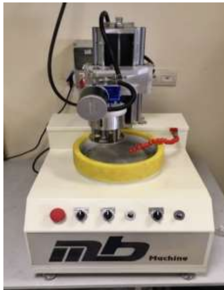
Figure 8: Grinding Polishing Machine after assembly
