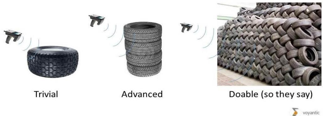
The use cases in tyre manufacturing, distribution, sales, usage and maintenance differ a lot. Reading a tag in a single tyre is relatively easy, even trivial, and does not pose high performance requirements from the tagging, because in most cases the read distance is short and nothing stands between the reader and the tyre.
