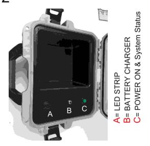
System SWITCH ON by Pushbutton C (Reset system by Pushbutton C off-on)
