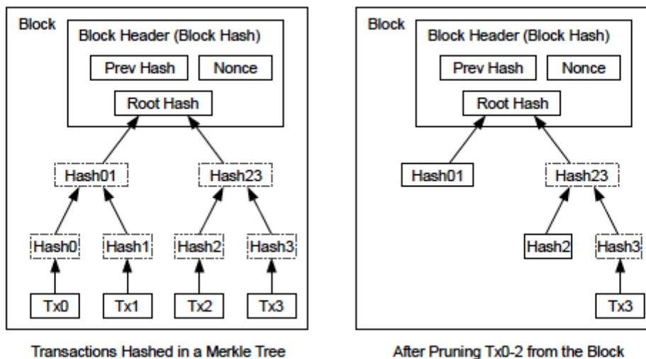
A block header with no transactions would be about 80 bytes. If we suppose blocks are generated every 10 minutes,  $80 \text{ bytes} * 6 * 24 * 365 = 4.2\text{MB}$  per year. With computer systems typically selling with 2GB of RAM as of 2008, and Moore's Law predicting current growth of 1.2GB per year, storage should not be a problem even if the block headers must be kept in memory.
