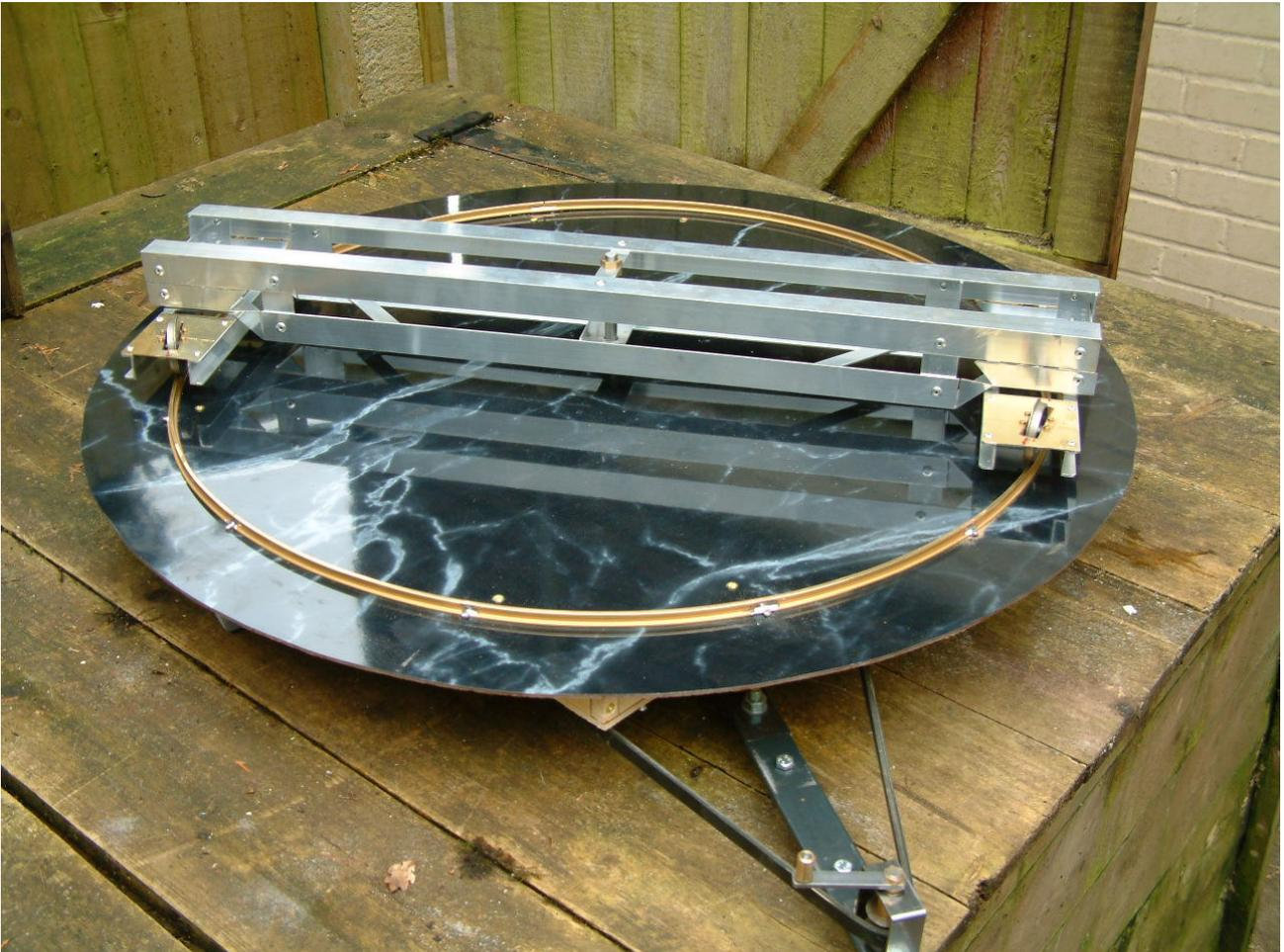
fixings for the turning mechanism and the supporting legs which hold the panel and the required level above the tank base. The latter requires a number of holes drilled around the edge to provide drainage.
