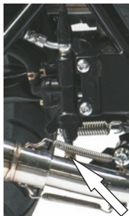
Adjusting push rod and lock nut.
