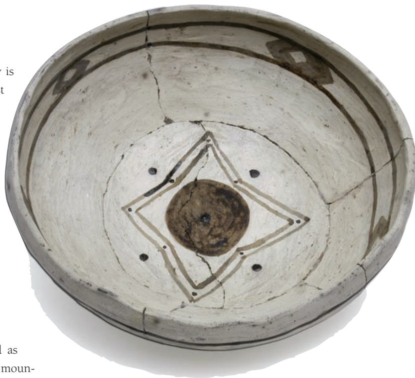
Learning by failure: a bowl by Joshua Madalena that “popped apart” in the fire because it did not have enough temper and was fired with too much heat, too fast.
