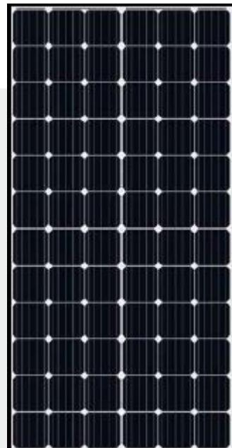
EXE high efficiency mono-crystalline 72-cell series grants high performance and conversion efficiency over 19,60%. This series features a 40 mm anodized aluminium frame, which combines robustness to light weight, and a 3.2 mm anti-reflective glass optimizing panel performance to solar irradiance. EXE monocrystalline cells are based PERC-technology and rear passivated.
