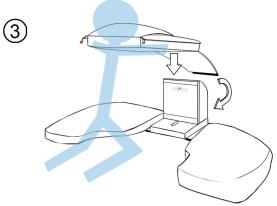
Carefully place & hold the roof and let it rest on top of the sound reducer.
