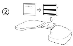
Attach the front to the Sound Reducer and place in line with the base-plate.
