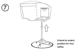
Lift the ISOVOX 2 and mount it on a PA-Speaker stand.
