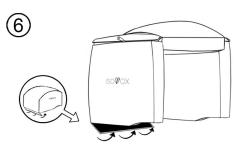
Also, attach the velcro side of the back flap on to the velcro stripe under the baseplate.
