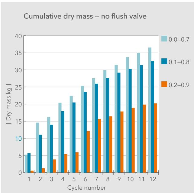
Figure 8. Cumulative mass of settling solids pumped out of the TOP sump in 12 pumping cycles for 3 operating stop-start level bands: 0.0-0.7; 0.1-0.8; 0.2-0.9
