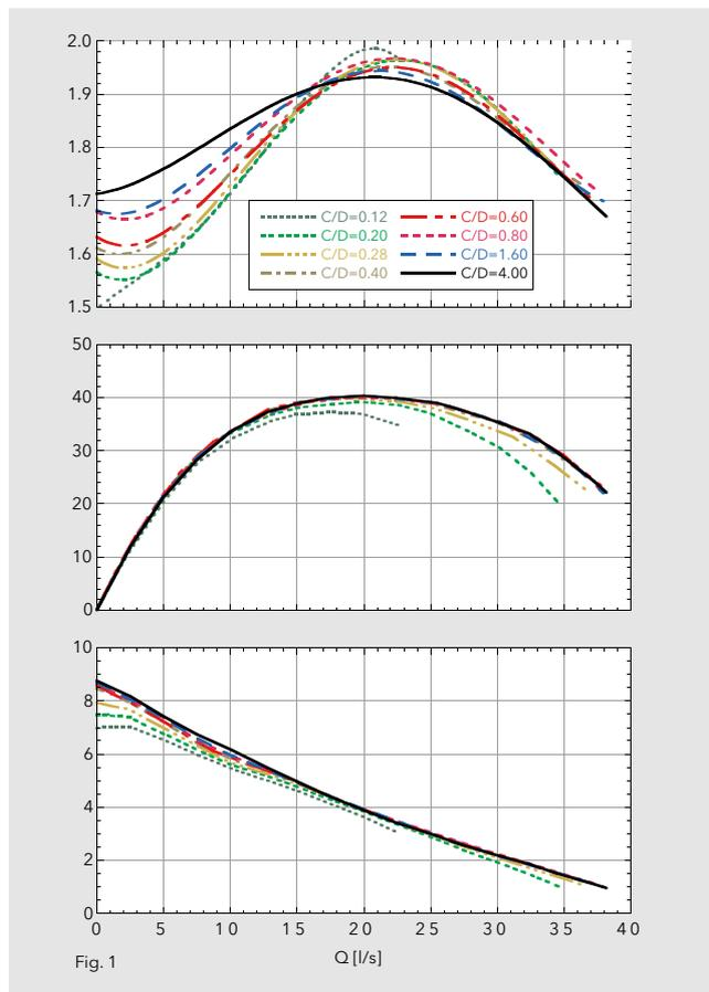
Figure 1. Effect of relative bottom clearance  $C/D$  on pump performance
