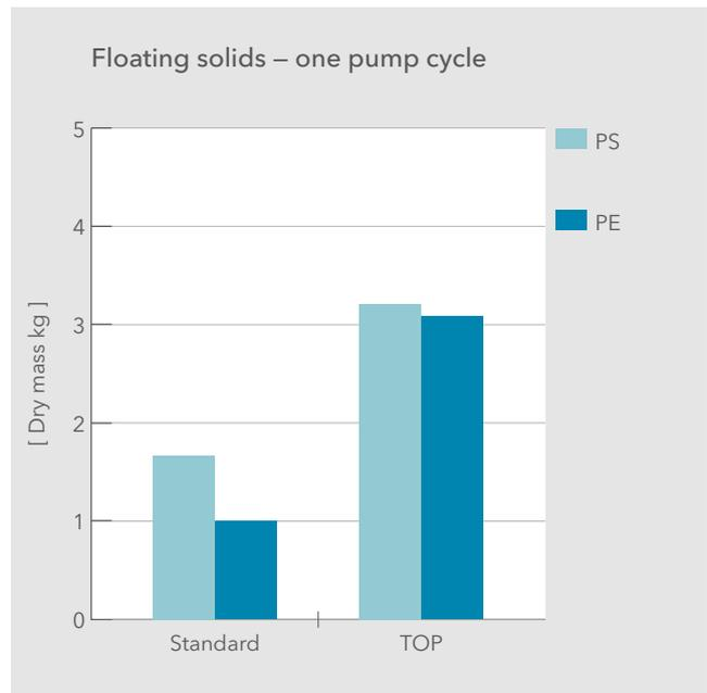
Figure 9. Mass of floating solids pumped out of the standard and TOP sumps in one pumping cycle; solids modeled by beads of polystyrene (PS) and polyethylene (PE)
