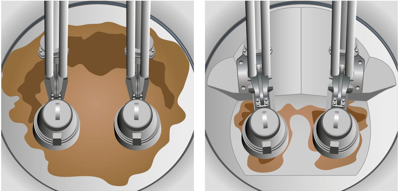
Figure 5. Back-to-back test - sand and plastic bead deposits (contour marked by a red line) in the standard and TOP sumps after a total of 40 pumping cycles. The mass of sediment in the standard sump was 94kg and in the TOP sump, 4kg
