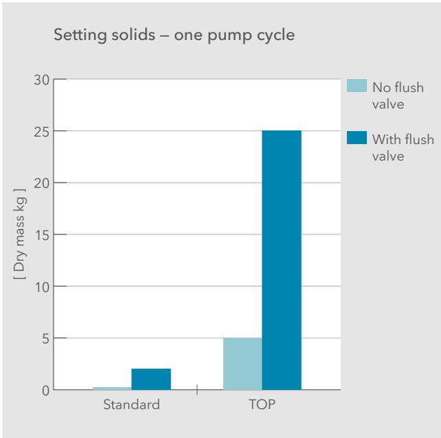
Figure 7. Mass of settling solids pumped out of the standard and TOP sumps in one pumping cycle
