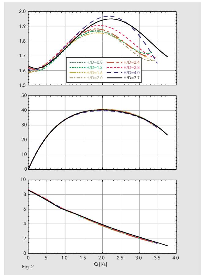
Figure 2. Effect of relative water depth  $H/D$  on pump performance
