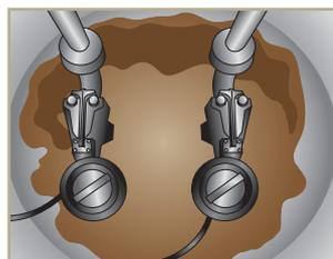
*The further away from the pumps, the greater the build up of sediment.*
