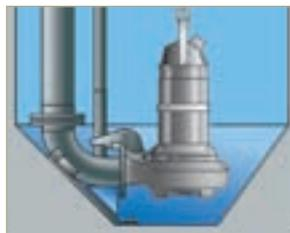
*The small floor and optimised geometries ensure high water velocity that whips settled solids into suspension.*
