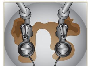
*Solids that are left behind will collect close to the pump, where the suction is the strongest. This means they will not have the chance to build up and stagnate.*
