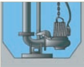
*It hasn't changed for over 30 years: a large flat sump floor that encourages the build up of sludge and solids.*
