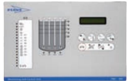
Fats and greases can be a problem in many sumps. APF is a supplementary controller that runs pumps down to the lowest possible water level. At this point, fat that's floating on the water surface is drawn into the pump. Also, at such a low water level a small amount of air enters the volute. This creates high turbulence, stirring up any remaining solids and fats.
