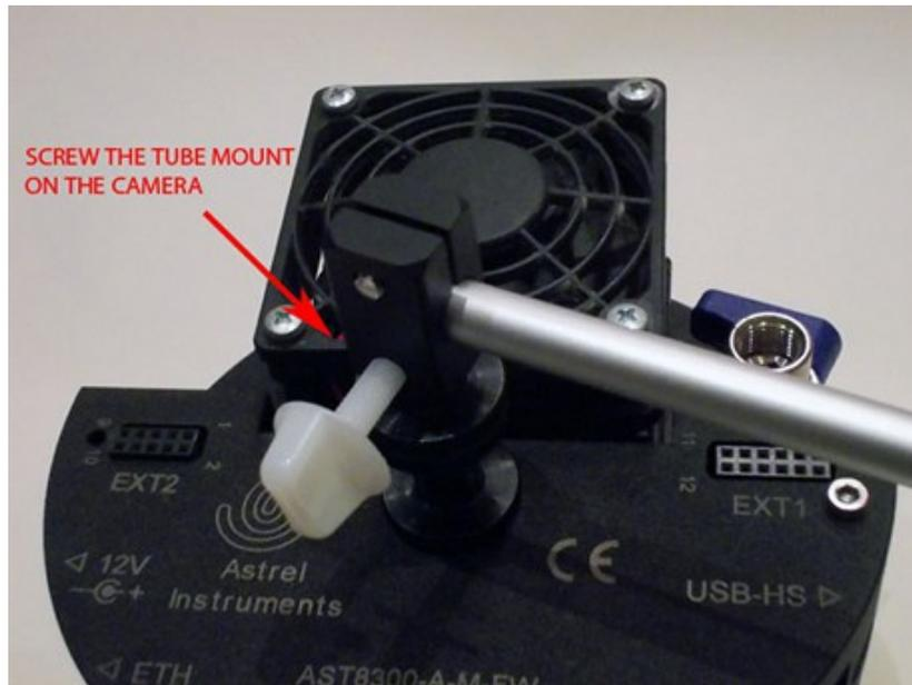
Mount the monitor as indicated in the pictures below: start by mounting the connecting tube to the back of the camera.
