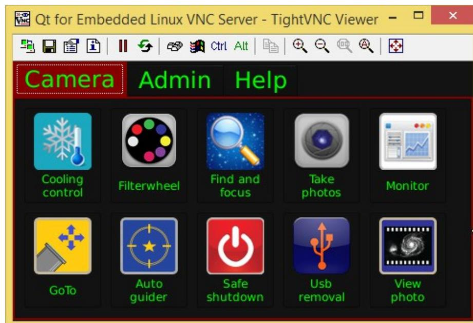
The camera automatically senses the presence of the touch LCD monitor at boot. When the monitor is not detected, the applications are started in VNC server mode and can be accessed by a VNC client.
