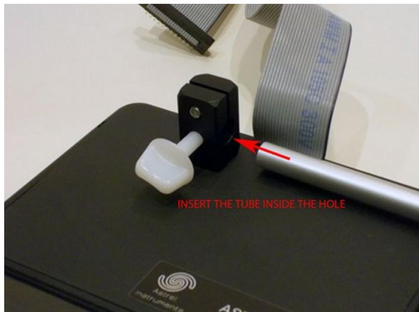
You can lock the monitor in the right position using the 2 white plastic knobs. Always be sure to lock the monitor properly to avoid movement during the exposures.
