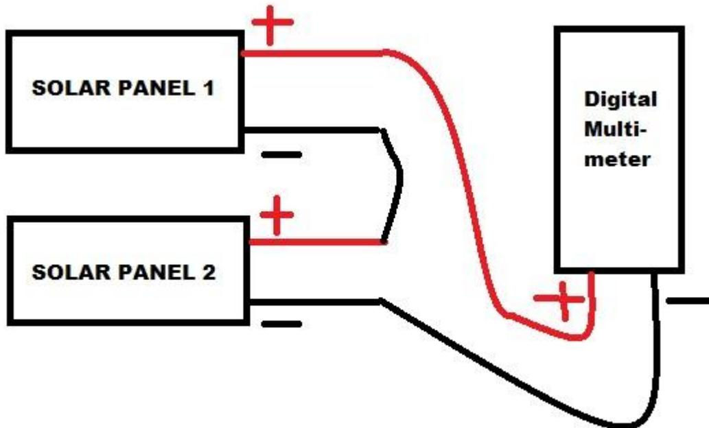
*Figure 1: PV cells in series*
