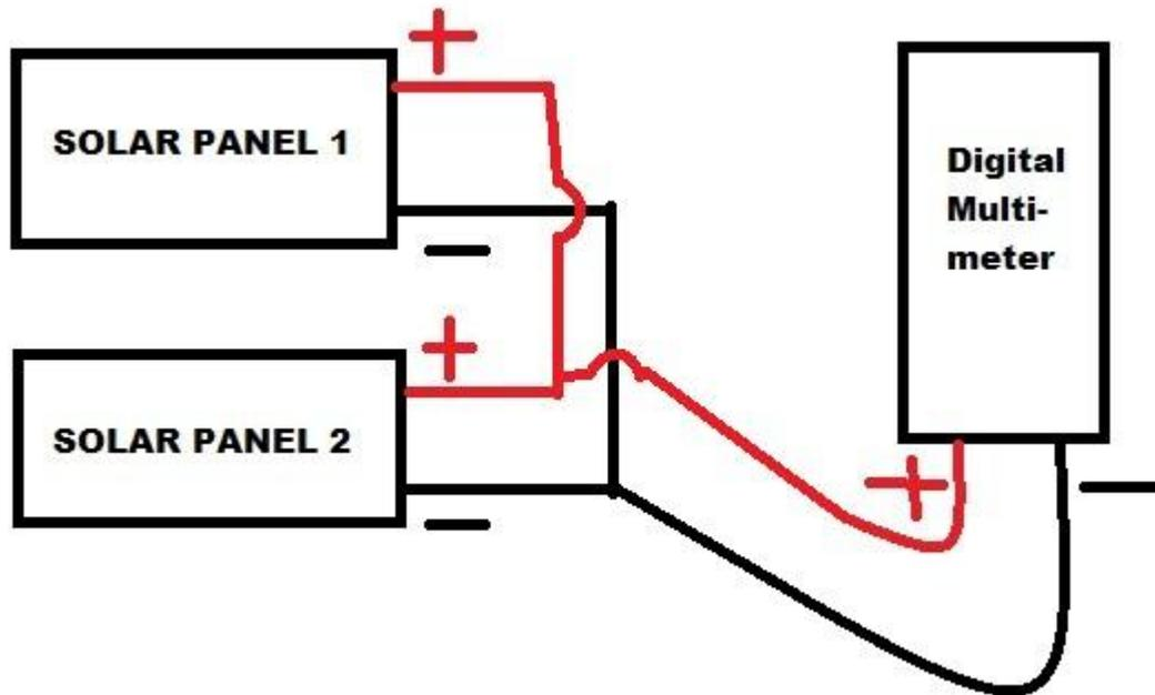
*Figure 2: PV cells in parallel*
