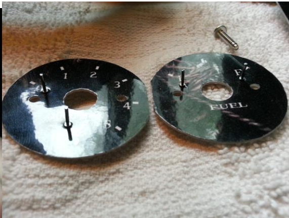
Step 8: Put the little metal pins in the new faceplate with a needle nose pliers.
