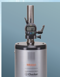
Inspection using digital indicator
