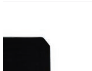
Chamfered part of a machined surface
