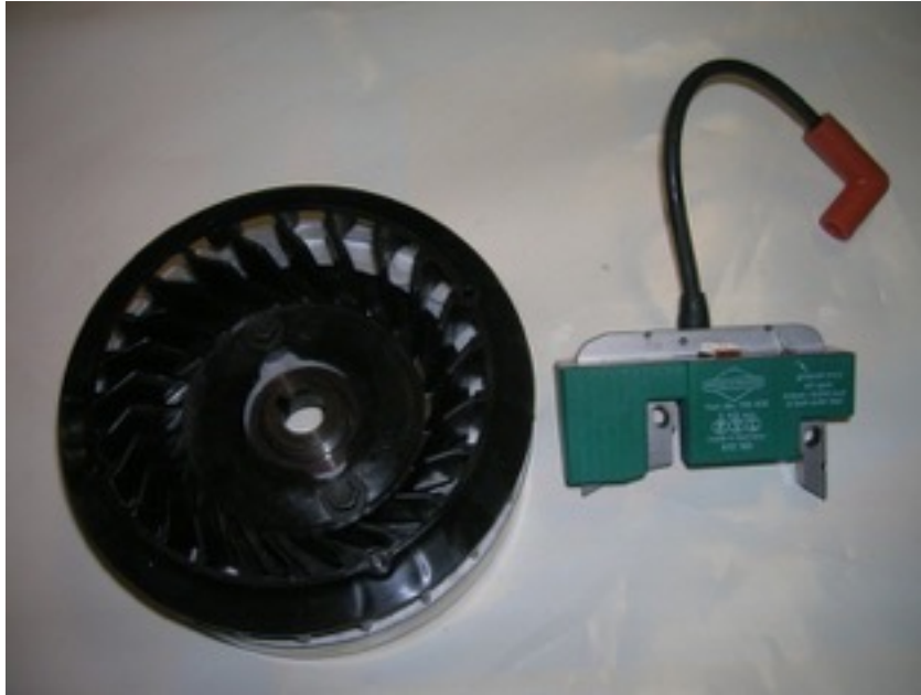
B&S PVL Ignition with Green Coil Max RPM 6100
