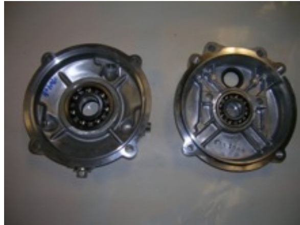
B&S 555721 Gear Reduction Box
