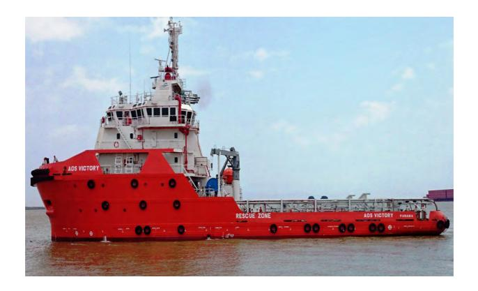
**AOS Victory** is a vessel equipped with two (2) Controllable Pitch Propellers and two (2) bow thursters and one (1) stern thruster. It is built of steel and engine room is located in the middle.
