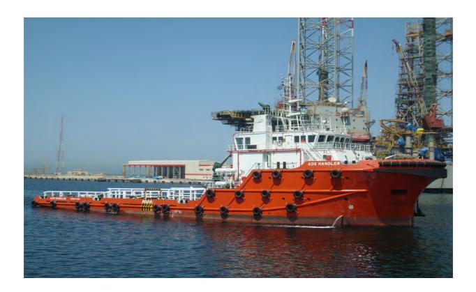
**AOS Handler** is a vessel equipped with two (2) Controllable Pitch Propellers and one (1) bow thruster. It is built of steel and engine room is located in the middle.
