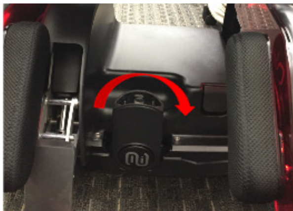
Figure 3 - Handlebar insert slot for steering control at base of device.
