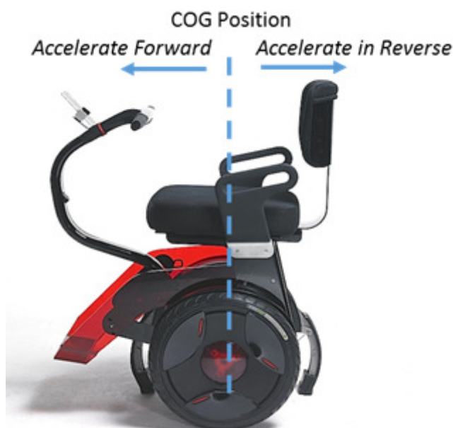
Figure 8 - COG and acceleration control of NINO smartchair.
