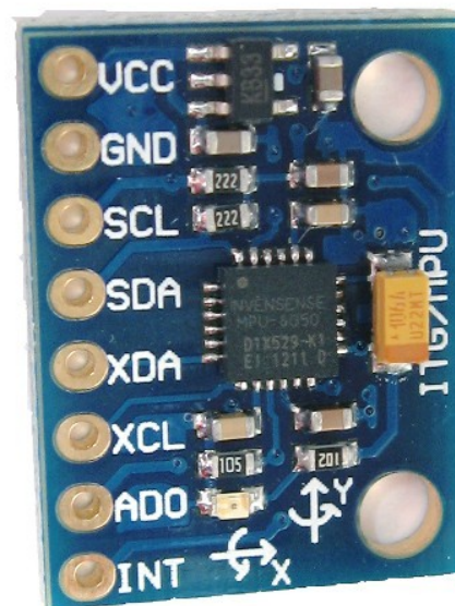
Figure 7 - InvenSense MPU-6050 accelerometer and gyroscope.
