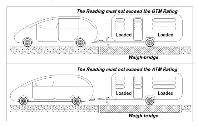
Drawing 1 shows measuring the "Axle-Loading" Must not exceed the GTM Rating
