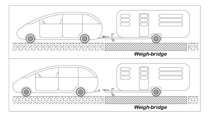
The Ball-Loading is the difference between the two readings
