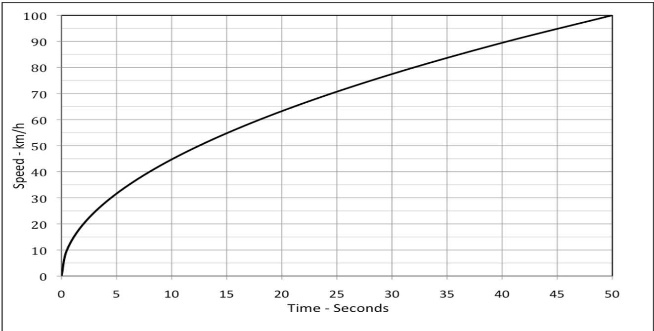
The graph shows the *inverted* typical “Acceleration Curve” for a combination.
