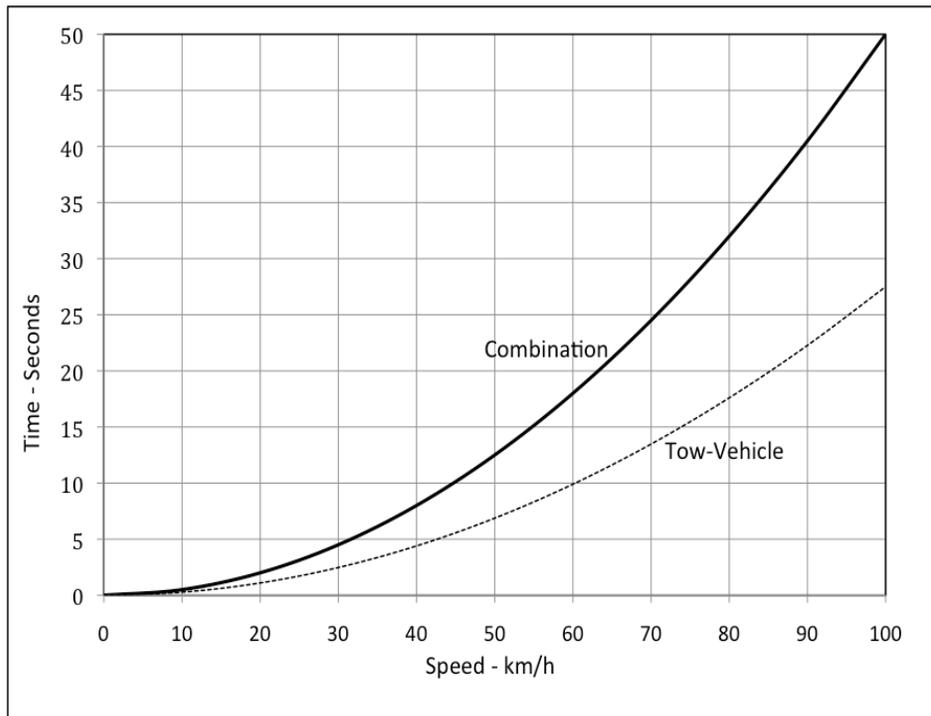
The graph shows a *typical* “Acceleration Curve” for an *average* (power and mass) car and caravan combination. The broken line shows a *typical* “Acceleration Curve” for just the tow-vehicle on its own.
