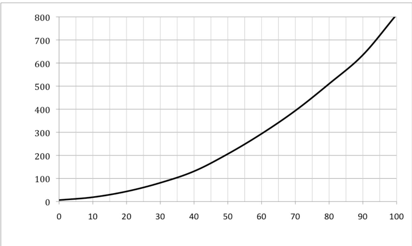
The graph illustrates a *typical* curve of “Distance covered V Speed” for an acceleration run, from a standing-start.
