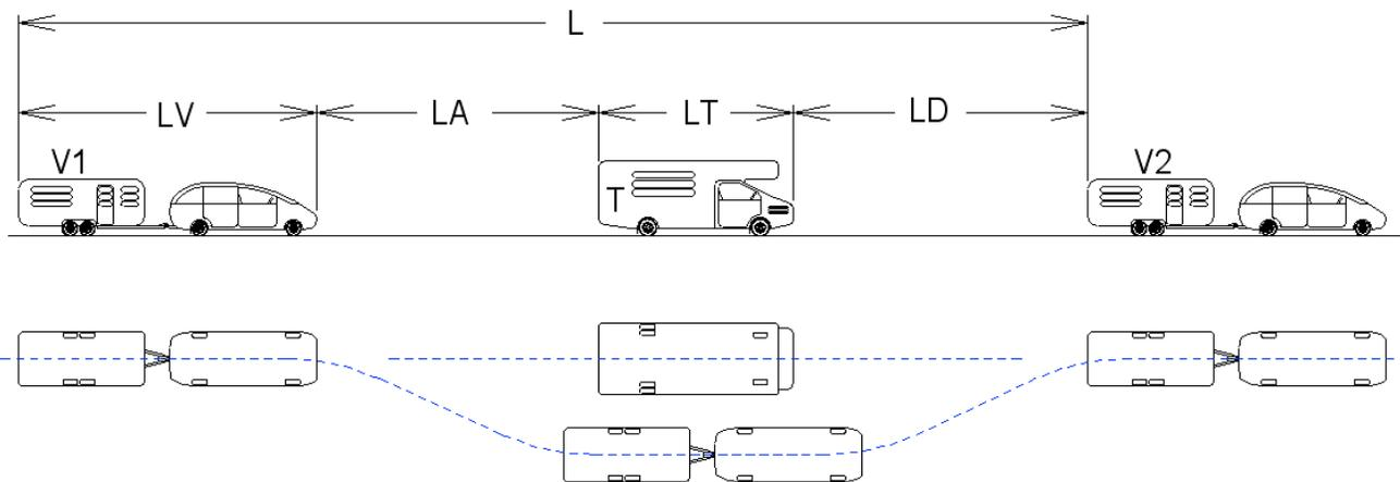
The drawing depicts a car-caravan combination [V1 & V2] over-taking another vehicle [T] (in side & plan views). The drawing is *not* to scale, as LA and LD are relatively *much* longer than LV and LT.
