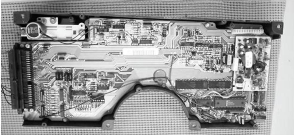
3. Remove the *seven (7)* 7/32" screws holding the Logic Board to the gauge unit.
