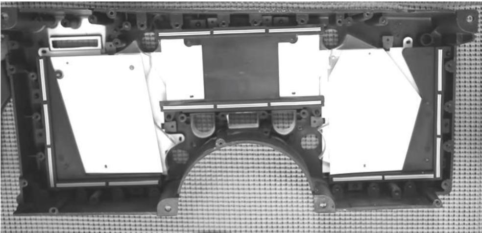
5. Remove the stencils and rubber blocks from the edges of the LED displays.
