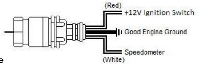
If you have a three-wire sender, you will need to contact your vehicle manufacturer to ask exactly which wire is the signal wire, as the wire colors can vary between manufacturers.
