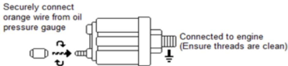
**Make sure** to test all fittings and connections for leaks. If any leaks are detected, determine the cause and repair immediately.
