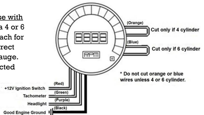
**The default setting for the tachometer is for an 8-cylinder engine.**
