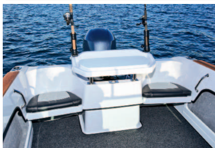
For fishing, the moulded fibreglass bait table slots into rod holders across the transom well. Rear corner seats lift out for better transom access.
