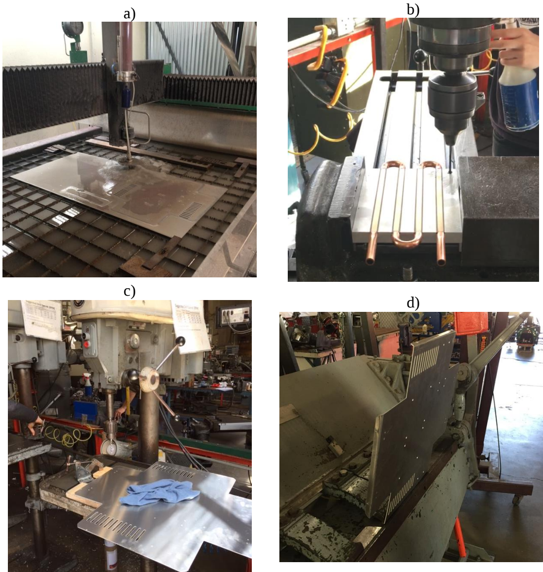
Figure 11. Our manufacturing process a) shows the water jetting of the sheet metal b) shows the drilling and tapping of the cold plates c) shows the post process drilling and deburring of holes in the sheet metal and d) shows the bending of the sheet metal
