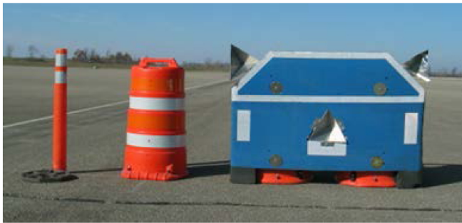
Figure 2. Final UMTRI fixed vehicle targets compatible with radar and vision systems
