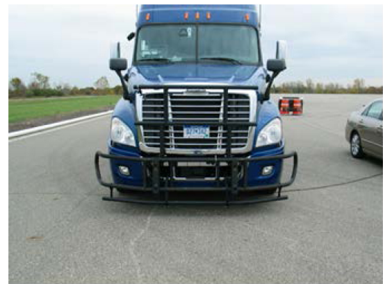
Figure 1. Subject vehicle with fabricated grill guard to protect against impacts with the target.
