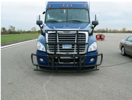
Figure 1. Subject vehicle with fabricated grill guard to protect against impacts with the target.
