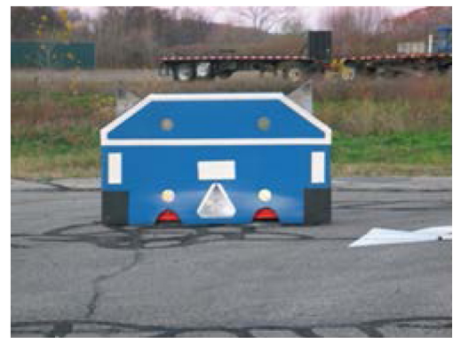
Figure 2. Final UMTRI towable target compatible with radar and vision systems
