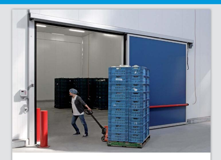
Door leaf constructed of a core of 100mm insulation material, covered on both sides with polyester and finished all round with anodized aluminium profiles, thermal bridge-free. Equipped with an aluminium drop/lift rail system.
