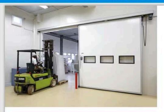
Door leaf constructed of a core of 40mm insulation material, covered on both sides with polyester and finished all round with aluminium profiles, thermal bridge-free. Equipped with an aluminium drop/lift rail system.
