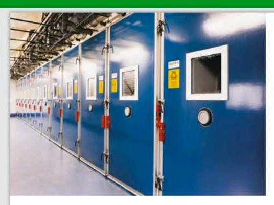
Door leaf constructed of a core of 100mm insulation material, covered on both sides with polyester and finished all round with anodized aluminium profiles, thermal bridgefree. Equipped with a 'lift and drop' hinge.
