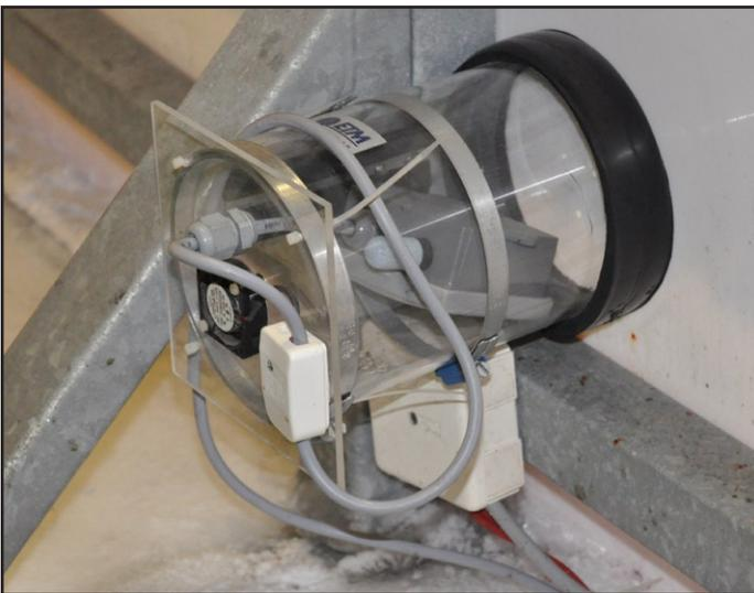
“In the ice hall, we measure temperature and relative humidity just above the surface of the ice, and temperature in the ice and in the concrete slab under the ice. We also monitor humidity elsewhere in the hall.”
