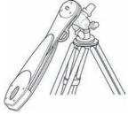
4. Adjust the tripod head so that the TT320X is angled for your latitude and the camera mount thread points approximately north.
