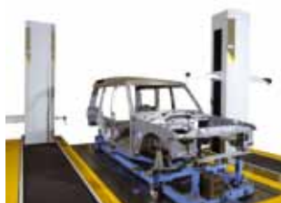
LK H-R dual column horizontal arm CMM
