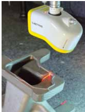
Scanning of casting
