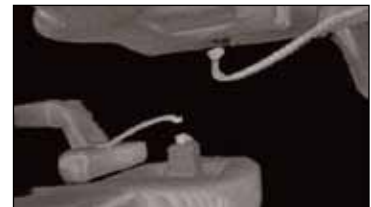
Damaged wirebond in IC
