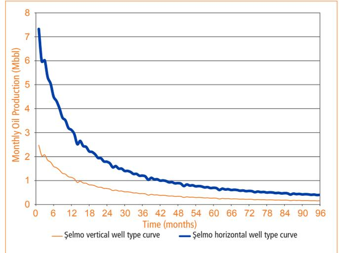
Figure 2. Comparison of vertical and horizontal wells type curves in Şelmo field.
