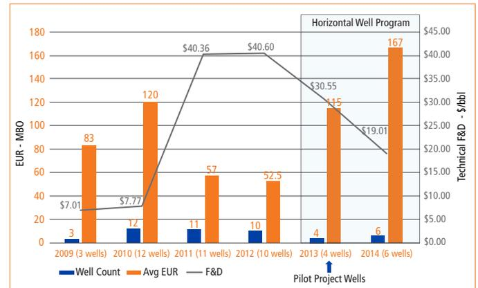
Figure 3. The diminishing returns of a vertical exploitation program as compared to horizontal multi-stage program in Turkey's Şelmo field.
