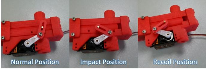
xxii. Once in position. Secure the servo horn (IT 7b) onto servo (IT 7a) using the retaining screw (IT 7d). xxiii. Assembly of the compact recoil unit is now complete.
