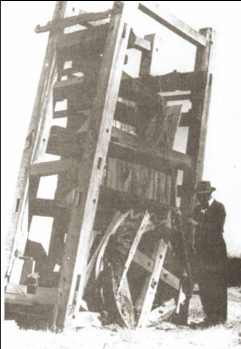
Hemp was a major crop of the area in the 1800's and a Hemp Press, above, was used to press the hemp into bales.
