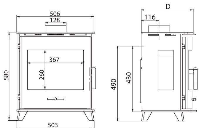
**40FS D = 338mm 50FS D = 377mm 60FS D = 434mm**
