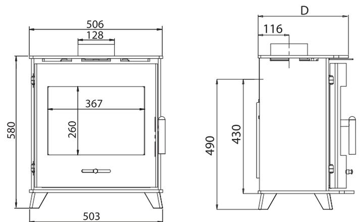
40FS D = 338mm 50FS D = 377mm 60FS D = 434mm
