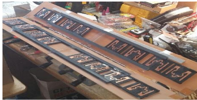
Figure 7.2. Dual fractal pattern of tri-pole arrays. Notice that the fractal pads slide on a channel, which uses a via and slide bar under the pad to adjust the fractal tri-pole arrays.
