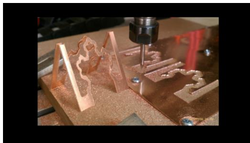
Figure 7.2. Dual fractal pattern of tri-pole arrays. Notice that the fractal pads slide on a channel, which uses a via and slide bar under the pad to adjust the fractal tri-pole arrays.
